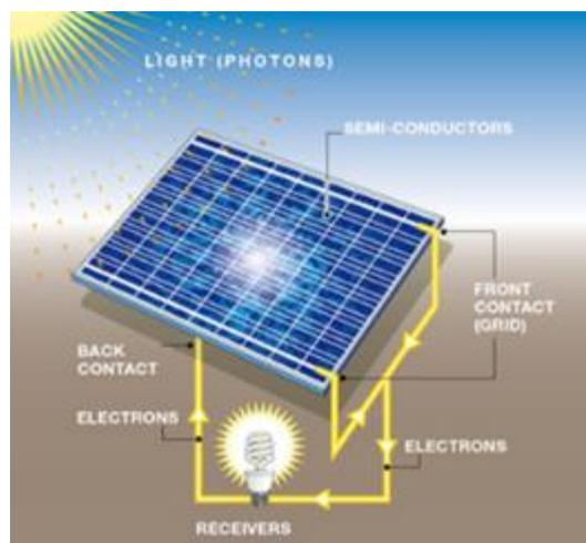
Figure 1: Schematic of a solar module connected to an electrical circuit (Source: Total.com).
