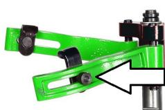
2. Place the spring between the inferior supporting arms (6) and turn the inferior lock nut clockwise:
