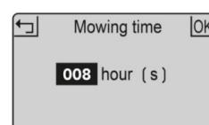
For example: if it is set to 8 hours and the robotic lawn mower is set to operate from 8:00pm, it will operate until 4:00am. In this time, it can operate for one hour, charge for two hours, mow again for one hour, charge for two hours, mow for one hour and charge again for the next cycle
