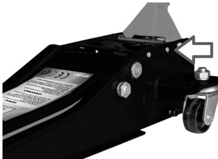
Remove the top plate and the oil filler plug:
