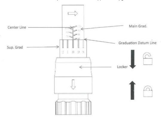
2.2 Turn the supplementary graduation handle to select the torque (combining the values of the main and secondary graduations).
