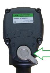
For reverse rotation, press the speed control knob on the left side of the tool.
