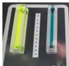
When the colour of new and used fluid is similar that means the exchange finished.
