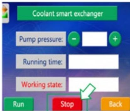
When the exchange finished, wait 30 minutes before removing the hoses.
