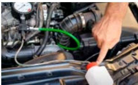
The maximum pressure limits it's of 1300 BAR. Start the engine and check the pressure to ensure its above 1050bar. If it's low, the pump or pressure regulator is faulty. Conduct a pump pressure regulator test to identify the issue. A pressure sensor issue on the fuel rail can cause the pressure regulator to open early, resulting in low pressure readings. Check the pressure using an EOBD tool with live data and compare the gauge pressure to the tool's reading.
