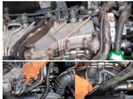
With fuel system de-pressurised, disconnect accessible high-pressure pipe and connect gauge with either M12 or M14 hoses. Make sure all hose fittings are tight before proceeding.
