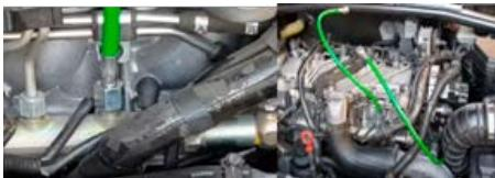
Connect a diesel waste bottle with a tube to the bottom of the gauge to collect waste fuel when the pressure relief valve is activated.
