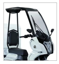
**Driver protection** Front screen and roof protects riders from cold rain and harsh sun. The wiper with a washer function ensures good visibility even in rainy weather.
