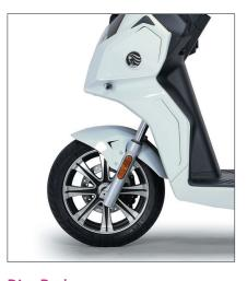
**Disc Brakes** Combination brakes (front and rear disc brakes) that link the front and rear to provide stable braking force.
