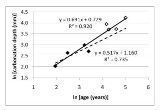
Figure 5 – Determining the exponent 'n' in the expression d = kt<sup>n</sup>
