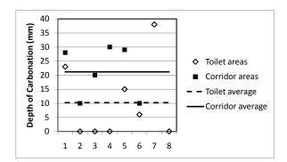
Figure 6 – Carbonation depths at Bandaranaike Wing, Colombo General Hospital
