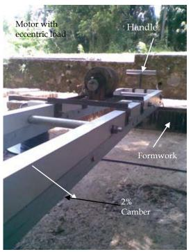
Figure 5 -Double beam surface vibrators
