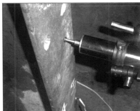
Figure 5: Displacement transducers in measuring displacement
