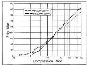
Figure 9: Comparison of two JPEG2000 codecs for edge blur against compression ratio.
