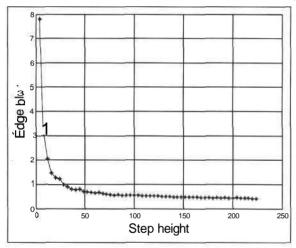
Figure 5: The variation of Edge blur with step height for a JPEG codec at qualityfactor of 20.
