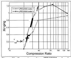
Figure 10: Comparison of two JPEG2000 codecs for ringing against compression ratio.
