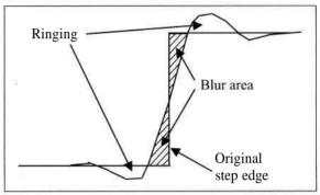
Figure 2. Ringing and edge blur at an edge of a onedimensional signal.
