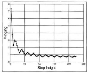
*Figure* 6: *The variation of ringing with step heightfor a JPEG codec at quality factor of 20.*
