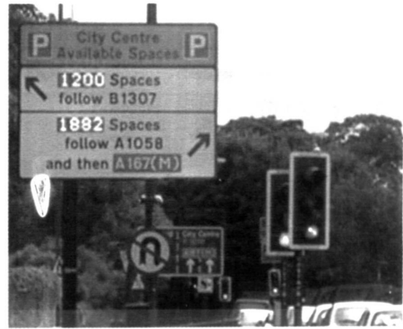
Figure 4: Variable message sign (VMS) to display the available spaces in Newcastle upon Tyne, England.
