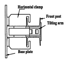
There is a diagonal bracing welded between the plate, which is welded at the gap between Cchannels, and the base plate. This diagonal bracing helps to transfer the vertical load applied on the tilting arm and flat plate to the base plate as a compression force. That is very important in the construction field, since the concrete can withstand much larger compressive forces.
