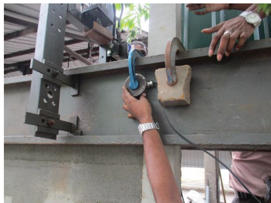
Figure 12 - Slip form Shutter Horizontal Force Measurement
