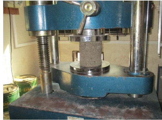
Figure 17 - Compressive Strength Test of Specimen Core Samples
