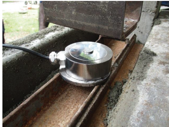
Figure 11 - Vertical Lifting Force Measured by Using Compressive Load Cell
