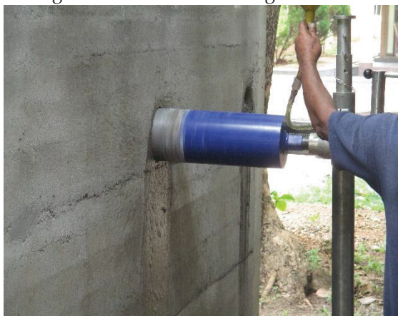
Figure 16 - Cylindrical Specimen Core Samples Cut by Machine
