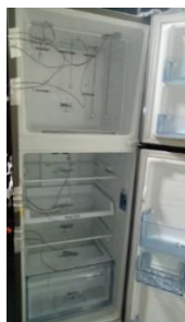
Figure 2 - Typical Picture of Temperature Sensors attached to Refrigerator Compartments
