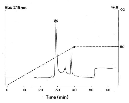
Figure 2: IIPLC separation of peptide 103. The gradient of acetonitrile (solvent B) is indicated by the broken line. Absorbtion was measured at 215nm and is given in arbitary units. Elution was performed at 10ml min<sup>-1</sup>. The peak containing peptide is indicated by an asterisk.
