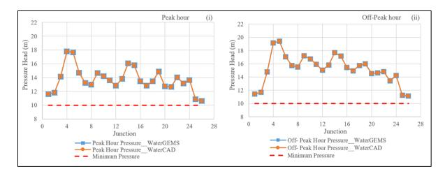
Figure 11: Pressure head vs elevation of nodal junctions (i) Peak, (ii) Off-peak hours
