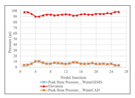
Figure 12: Pressure head vs elevation of nodal junctions
