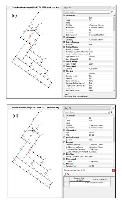
**Figure 3**: The procedure of (a) creating the model, (b) water tank data input, (c) pipes data input, and (d) nodal data input
