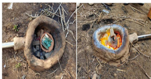
Fig. 4 Experiment 3 process (a) Process of bronze melting in crucibles with a special-shaped crucible
