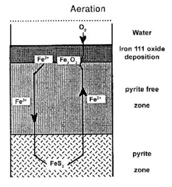
**Figure 4.**Model of pyrite oxidation in shrimp culture ponds constructed using acid sulphate soils.
