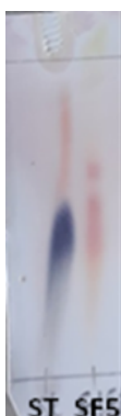
Figure 1. TLC analysis of ethyl acetate fraction of SF5 endophytic fungal extract of M. pruriens plant (The left most spot in the TLC plate was of the standard L-Dopa-carbidopa)
