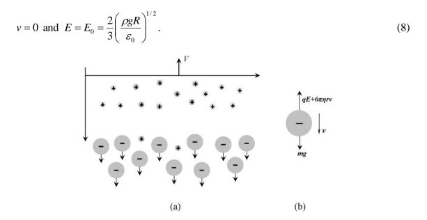
**Figure 2:** (a) Schematic diagram illustrating motion of graupel with a velocity *v* relative to the updraft moving with a velocity *V* relative to the earth (b) forces acting on a particle of graupel.
