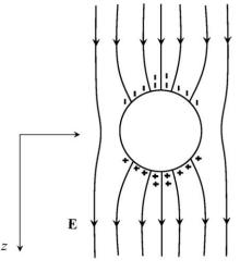
Charge carried by falling graupel per unit time per unit area is NQv, where N is the number of graupel particles per unit volume. Assuming that the field *E* generated is similar to a parallel plate capacitor we obtain,
