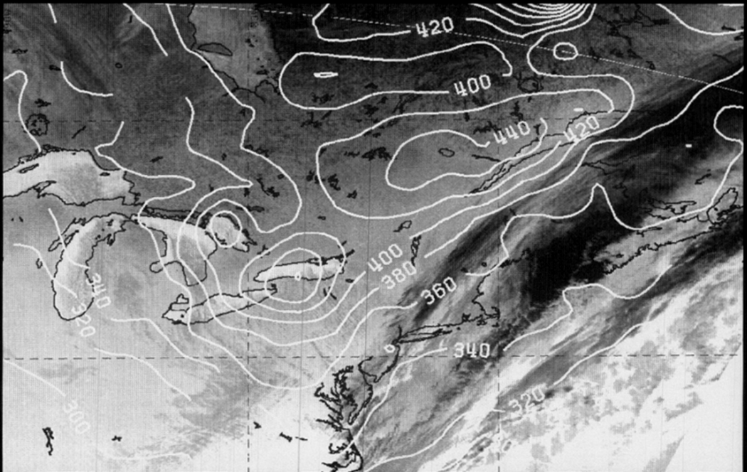
Fig. 8. An AVHRR channel 4 infrared image from 13:05 GMT, 29 February, with TOVS column ozone contours overlaid.
