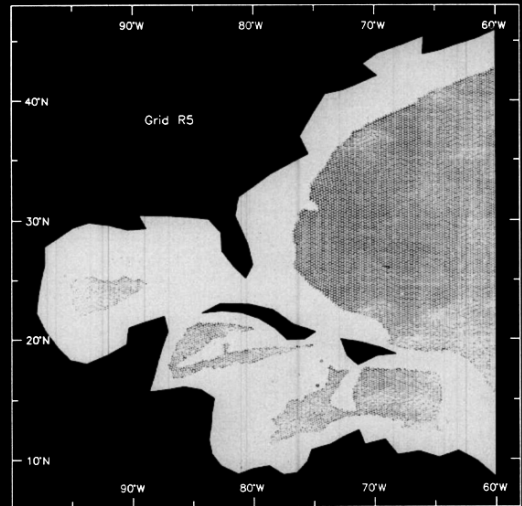
Fig. 4. Grid R5. Nearly regular finite element 6' \times 6' to 12' \times 12' discretization of the domain with a coarse representation of the coastal boundary.
