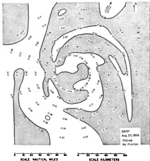
FIG. 20. Non-dimensional vertical velocity field for Hurricane Daisy. The results apply for the case y = y_1 , where none of the friction terms are included. To obtain the vertical velocities in units of millibars/hour, multiply by 131.22.
