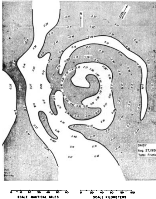
FIG. 22. Non-dimensional vertical velocity field for Hurricane Daisy. The results apply for the case y = y_1 + y_2 + y_3 + y_4 , where all of the friction terms are included. To obtain the vertical velocities in units of millibars/hour, multiply by 131.22.
