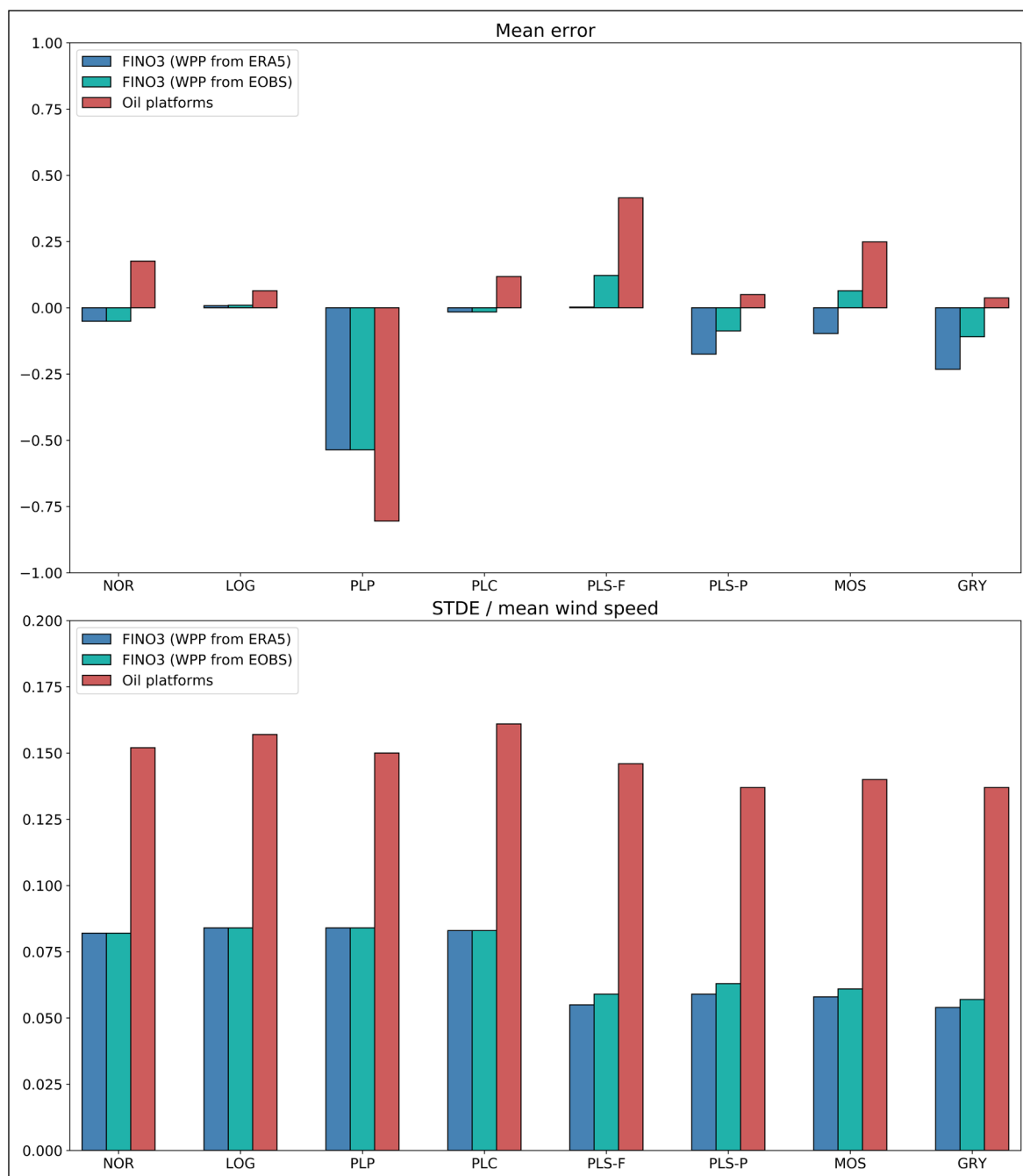
Figure 5 Mean error (ME) (upper panel) and standard deviation of the error (STDE) normalized by the mean wind speed (lower panel) for the five wind profile methods (with four different versions of the power law profile: PLP, PLC, PLS-F and PLS-P). At FINO3 wind profiles are calculated by using Wind Profile Parameters (WPP) based on both ERA5 and observations.
