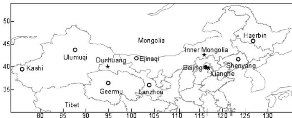
Fig. 1. AERONET sites (stars) and radiation sites (circles) over North China used in this study. The Cimel sun/sky radiometer in Beijing is installed on the top of Institute of Atmospheric Physics Building (in a northern suburb); the pyrheliometer in Beijing is installed at Beijing Meteorological Observatory (in a southern suburb). The two sites are about 40 km apart. Xianghe is about 100 km from Beijing.
