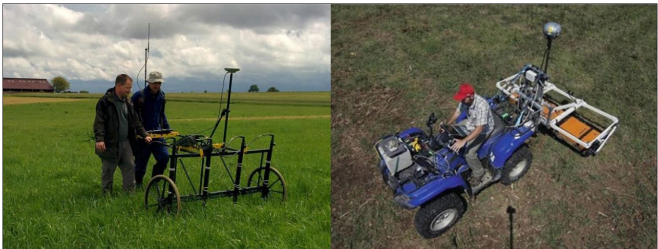
Figure 1: Multi-sensor array geophysics in action. Left: magnetic gradiometry, right: multichannel GPR survey (image courtesy Alexandre Novo and Geostudi Astier).
