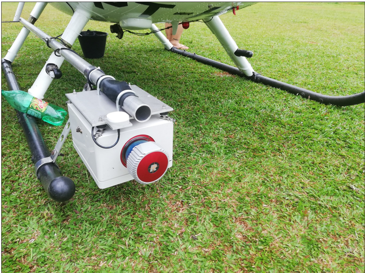
Figure 4: VUX-1 integrated into the Bell 500M helicopter.
