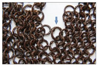
**Figure 5:** Larger riveted ring among regular sized ones. The larger rings are probably repairs made in antiquity. Photograph MA Wijnhoven.
