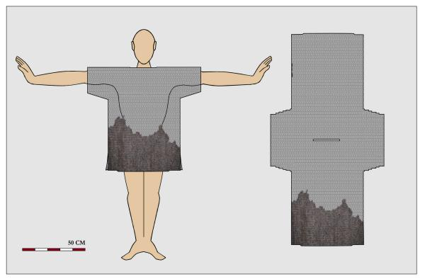
**Figure 12: Left:** The construction plan of the coat of mail in relation to the large fragment. Note that the majority of the fragment belongs to one side and only a small section comes from the other side. **Right:** Original location of the large fragment in the coat of mail (with left split and entire hem restored). Drawing MA Wijnhoven.
