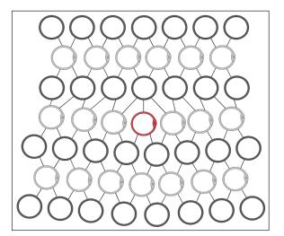
**Figure 16:** Representation of the use of an idle link to change the number of rings in a row. Drawing MA Wijnhoven.
