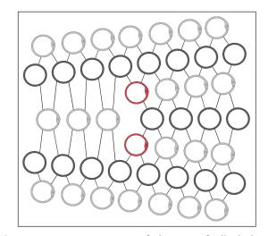
**Figure 17:** Representation of the use of idle links to change the number of rows. There are two manners in which idle links can be employed to this aim; one leaves a small hole, the other a knot. The former is illustrated here. Drawing MA Wijnhoven.
