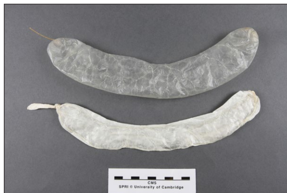
Figure 7: Comparing sausage skin which has been air dried (top) as opposed to freeze dried (bottom). Freeze drying resulted in a more opaque and silvery appearance. Photo: ©Scott Polar Research Institute, University of Cambridge.
