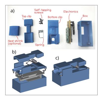
Figure 7 a) Finger clip components prior to Assembly.b) An exploded render of the assembly. c) A render of the assembled finger clip.
