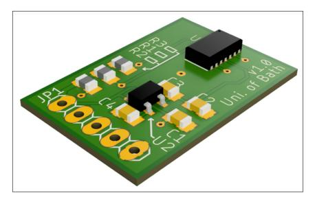
Figure 4 MAX3010x breakout board, developed as a dropin replacement in case of commercial breakout board supply shortage.
