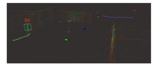
**Figure 14** Pedestrian detection and tracking output from RViz.
