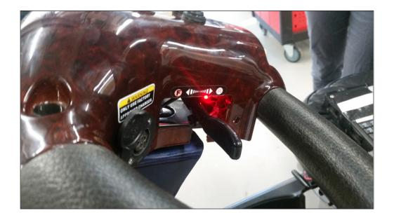
**Figure 12** Steering console showing the newly added relay (with lit LED).
