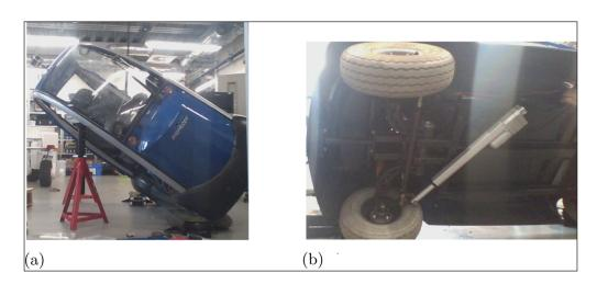
Figure 1 Vehicle mechanical modification. (a) Tilting the vehicle using two axle stands, to enable access to the underside. (Note also lidar mounted to roof.) (b) Underside with linear actuator added for steering.
