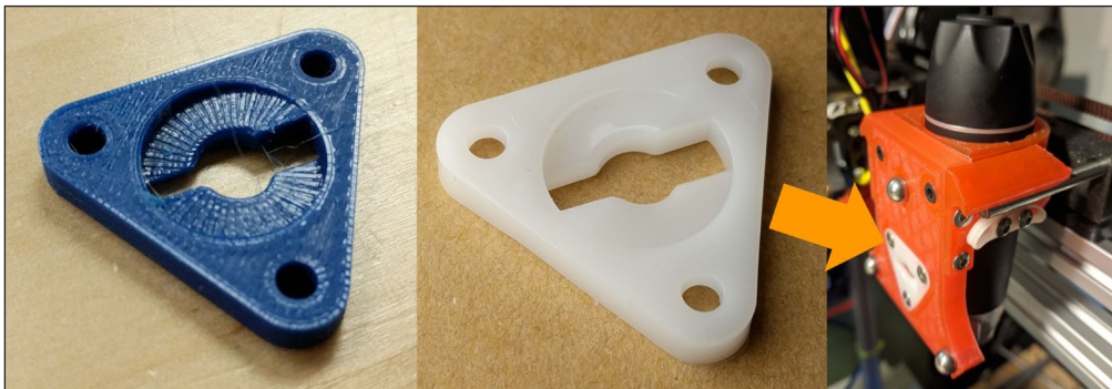
Figure 3 Left: the original 3D printed Wedge Plate. Center: the latest revision of the injection molded Wedge Plate after months of community experimentation. Right: the location of the Wedge Plate on the back of an example tool (a USB microscope). Note that the distinct lack of 'stair-stepping' dramatically improves the reliability of the tool's locking behavior.
