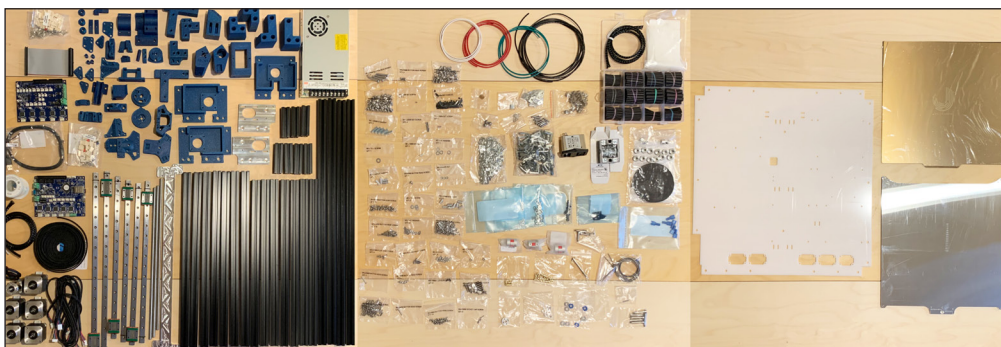
Figure 2 Jubilee's design comprised many separate parts to be sourced and assembled. Shown is a spread of the 800+ components needed for the motion platform (frame) of one Jubilee machine.
