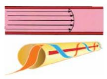
Figure 1. Two-dimensional versus threedimensional representation of laminar flow in a tube.
