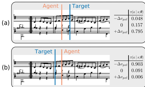
Figure 8: Two examples of policy outputs. (a) Agent is behind the target, resulting in a high probability for increasing the pixel speed ( \pi(+\Delta v_{pxl} | s; \theta) = 0.795 ). (b) Agent is ahead of the target, suggesting a reduction of pixel speed ( \pi(-\Delta v_{pxl} | s; \theta) = 0.903 ).
