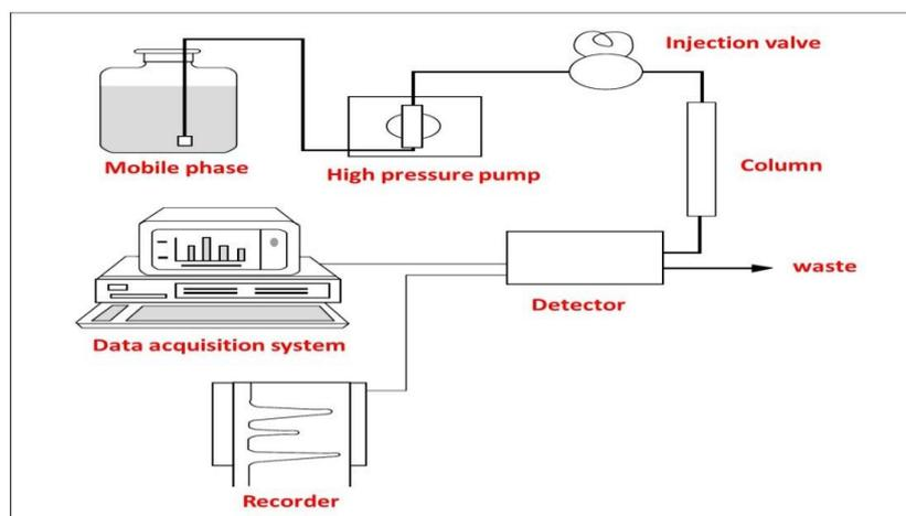
Figure 8. Schematic representation of an HPLC system.
