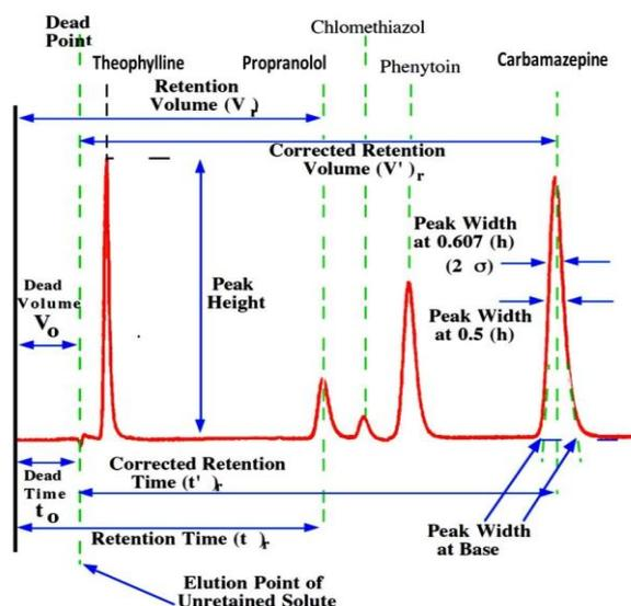
Figure 6. Parts of a chromatogram
