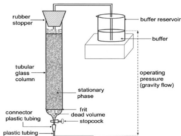
**Figure 5. Components of column chromatography**
