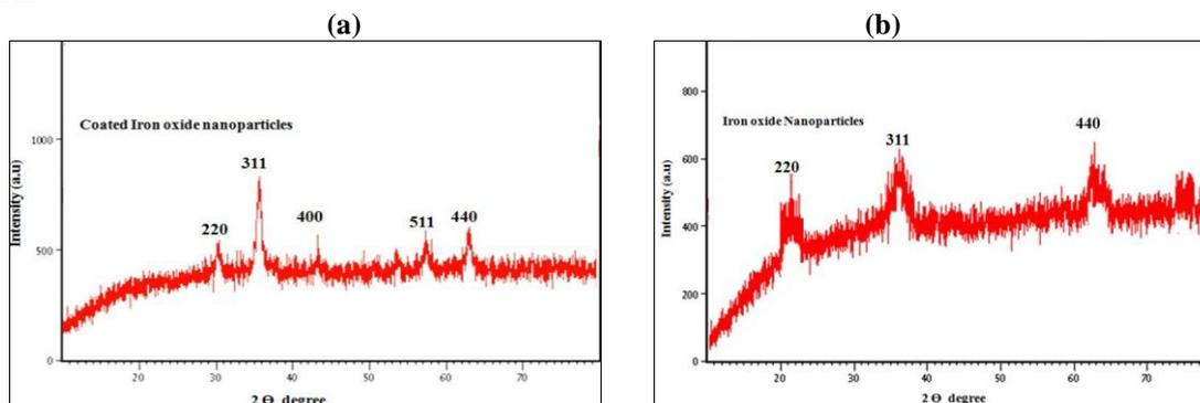
**Fig 5: XRD analysis of iron oxide nanoparticles (a) synthesised iron oxide nanoparticles (b) anethole coated iron oxide nanoparticles**
