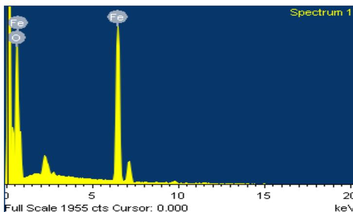
**Fig 4 : EDX spectrum of synthesised iron oxide nanoparticles**
