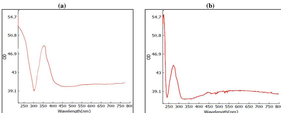
**Fig 1:** UV-Visible spectrum of iron oxide nanoparticles (a) synthesised iron oxide nanoparticles (b) anethole coated iron oxide nanoparticles
