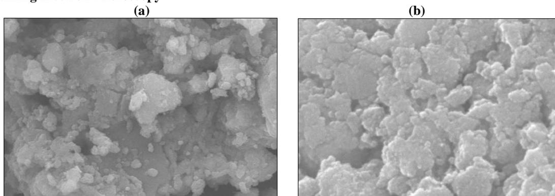
**Fig 3: Scanning Electron Microscopy of iron oxide nanoparticles (a) synthesised iron oxide nanoparticles (b) anethole coated iron oxide nanoparticles**
