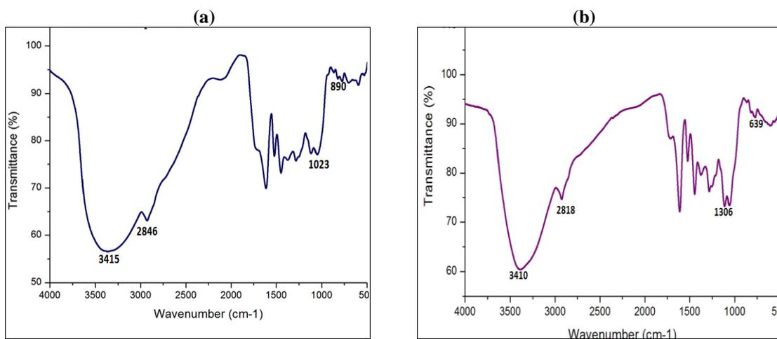
**Fig 2:** FTIR spectrum of iron oxide nanoparticles (a) synthesised iron oxide nanoparticles (b) anethole coated iron oxide nanoparticles
