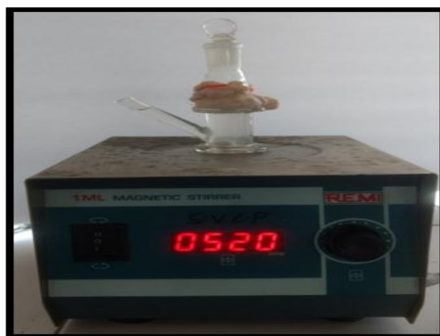
Fig-11 Franz diffusion cell along with magnetic stirrer.
