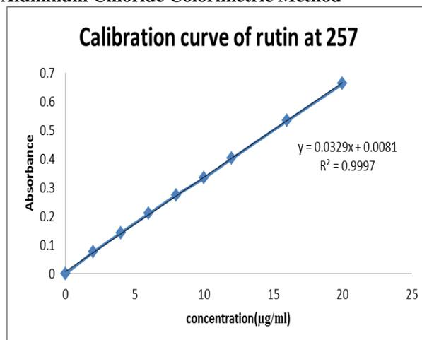
Fig: Calibration curve of rutin.
