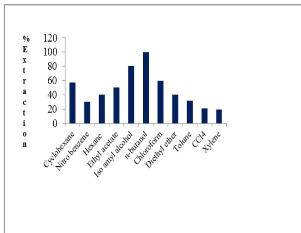
Fig. 1: Effect of solvent on extraction.
