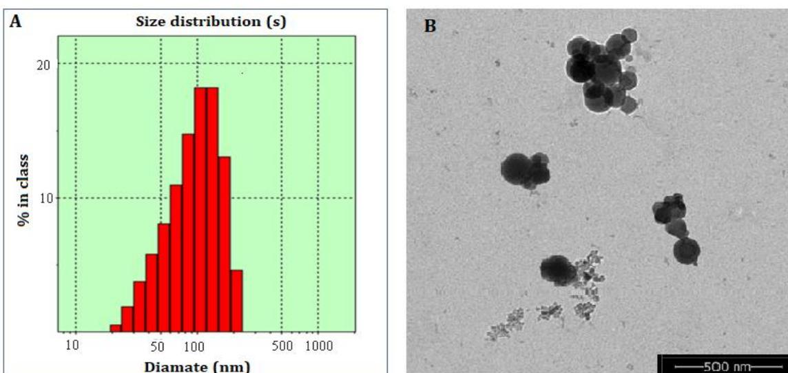
**Figure 5:** DLS and TEM characterization of PEG-HA-MEL. A: DLS characterization of PEG-HA-MEL. Particle size distribution of PEG-HA-MEL; B: TEM characterization of PEG-HA-MEL, the particle size is around 120nm, and the morphology of micelles is spherical.
