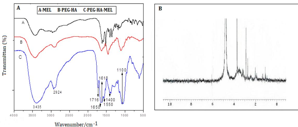
**Figure 4:** General procedure for preparation of PEG-HA-MEL Micelles. A: the FTIR spectra of MEL, PEG-HA and PEG-HA-MEL; the <sup>1</sup>H NMR B: spectrum of the micellar solution of PEG-HA-MEL.
