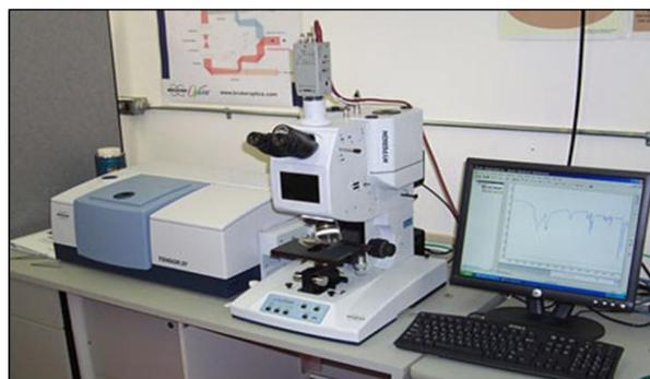
Figure 1: Ftir Instrument.
