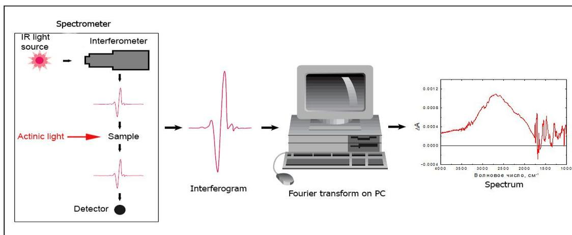
Figure 2: Ftir Mechanism.
