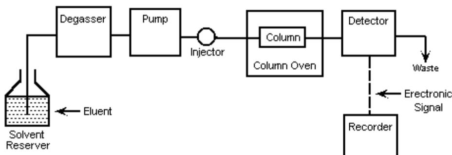
Figure 2: Components of HPLC system.
