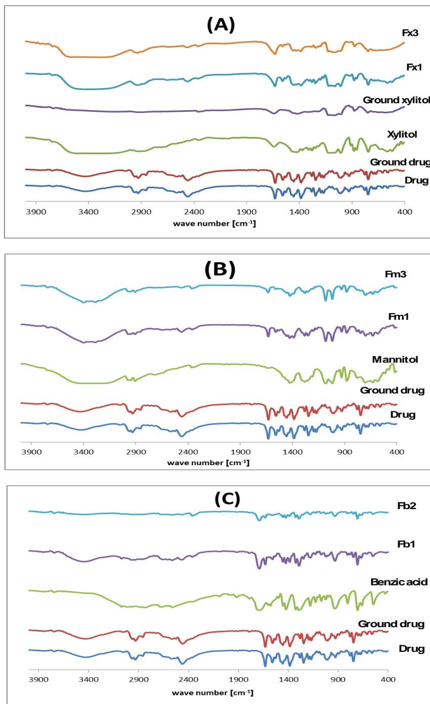
**Figure 1: FTIR spectra of amiodarone from different co-ground formulations prepared using, xylitol (A), mannitol (B) and benzoic acid (C). Detailed formulations are shown in Table 1.**
