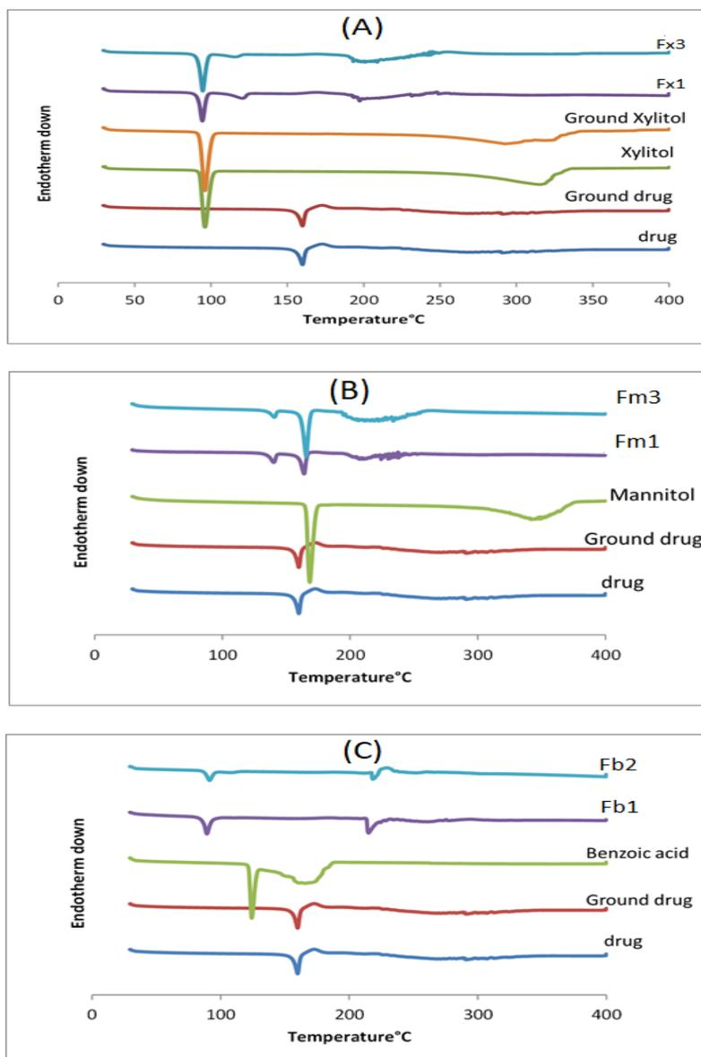
**Figure 2: DSC thermograms of amiodarone from different co-ground formulations prepared using, xylitol (A), mannitol (B) and benzoic acid (C). Detailed formulations are shown in Table 1.**
