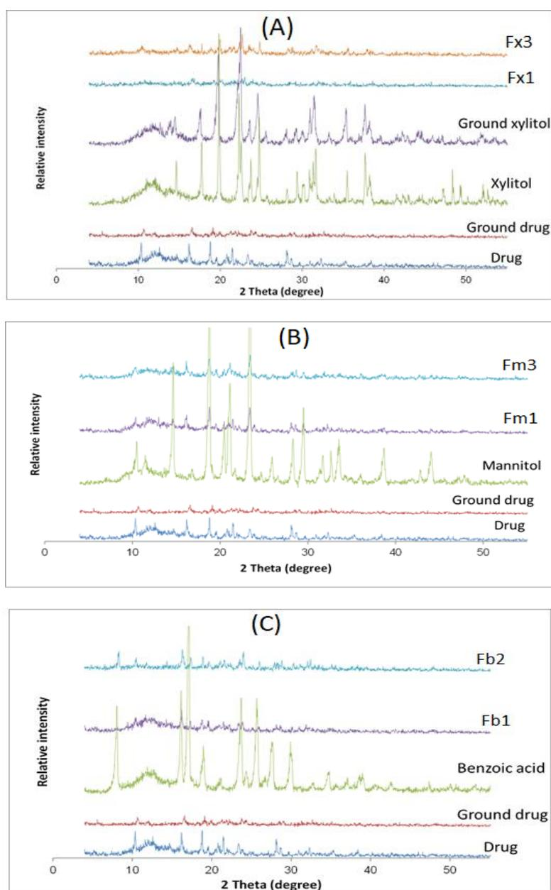
**Figure 3: Powder X-ray diffractograms of amidarone from different co-ground formulations prepared using, xylitol (A), mannitol (B) and benzoic acid (C). Detailed formulations are shown in Table 1.**
