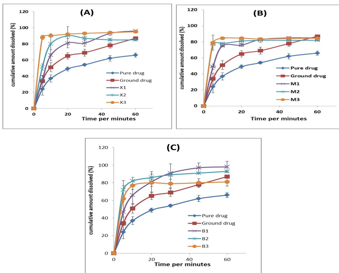
**Figure 4:** *In vitro* dissolution profiles of amiodarone from its pure and ground form and different formulations prepared using xylitol (A), mannitol (B) and benzoic acid (C).
