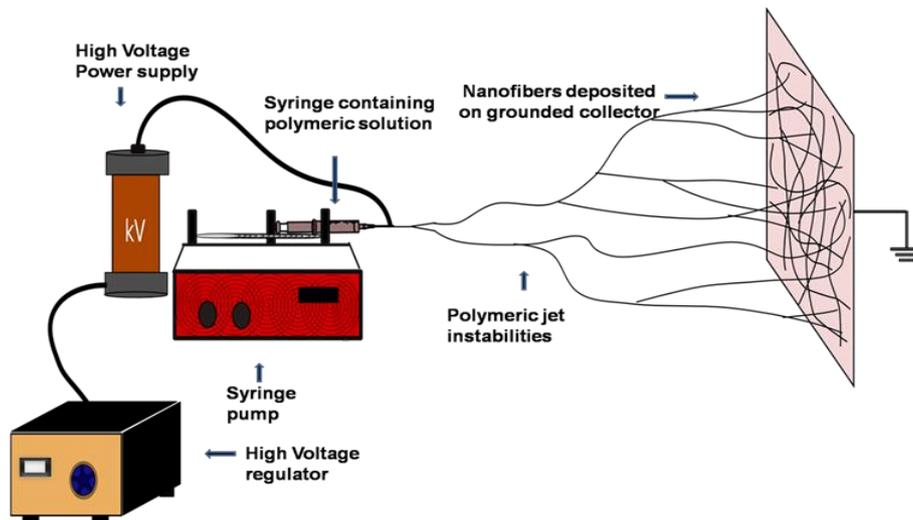
Figure 1: Electro spinning.
