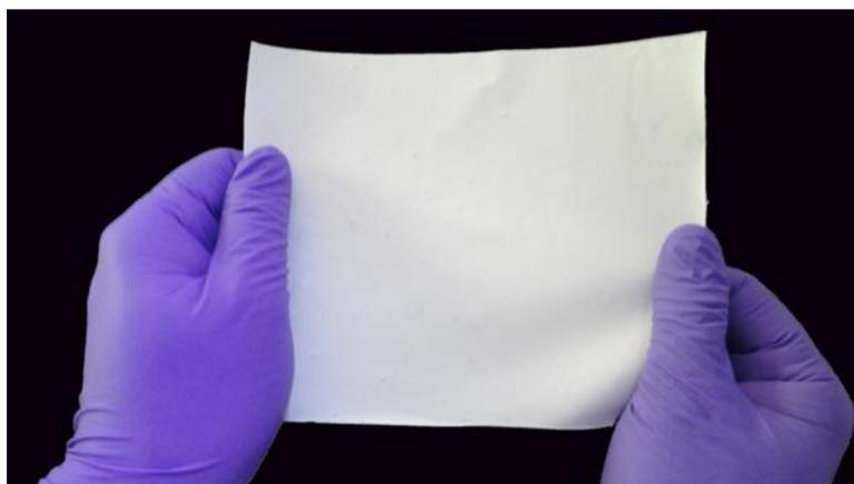
Figure 2: Electro spun PHBV Nano fibrous Mat.
