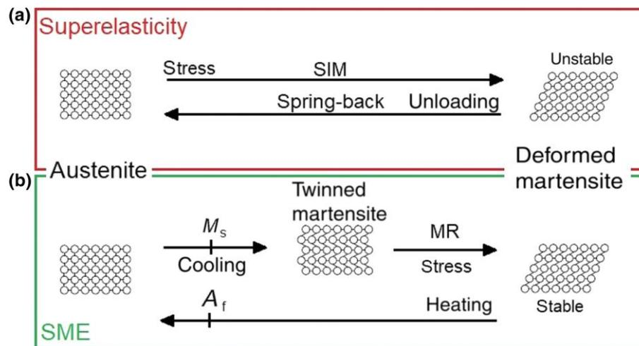
**Figure 1: Martensitic transformations. (a) Superelasticity (SE) at ambient temperature above austenite finish temperature (A). (b) Shape memory effect (SME). For the martensite reorientation (MR), less stress is required than for stress-induced martensite (SIM) transformation. ( $M_s$  = martensite start temperature).**
