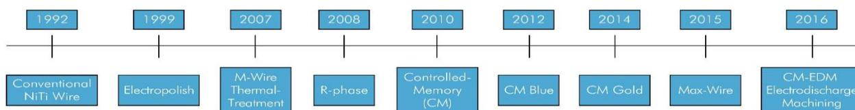
**Figure 3: Evolution of NiTi Alloy Treatments.**
