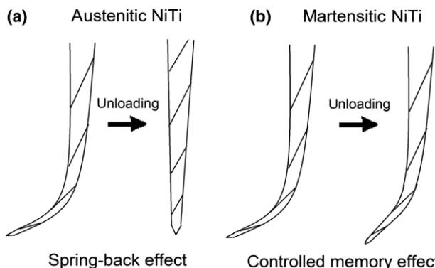
**Figure 4 (a): Spring-back effect of austenitic NiTi alloys (b) controlled memory effect of martensitic NiTi alloys.**
