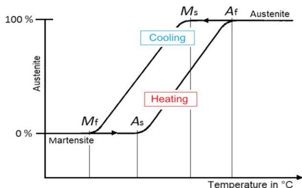
**Figure 2: Temperature hysteresis diagram of NiTi alloy. (M) martensite start temperature, (M) martensite finish temperature, (A) austenite start temperature, (A) austenite finish temperature.**
