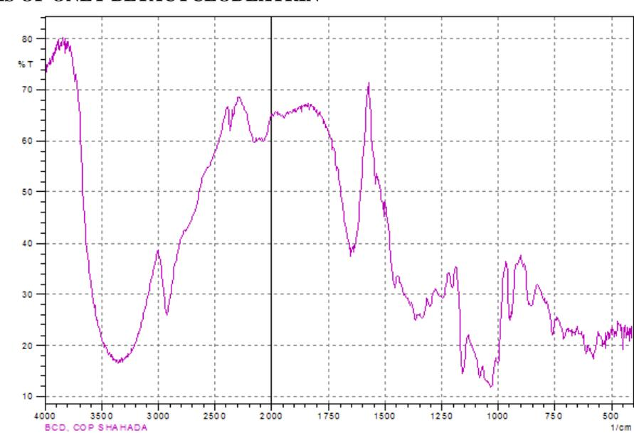
**Figure no 3: FTIR Spectrum of Betacyclodextrin.**
