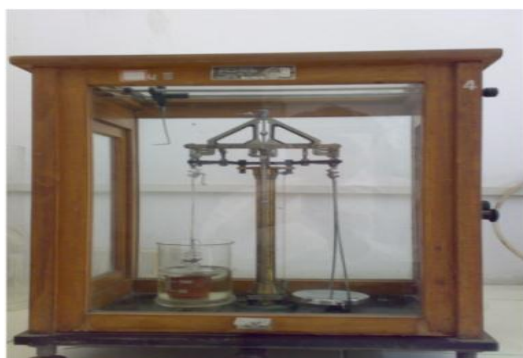
Figure 1: Modified physical balance for mucoadhesive studies.
